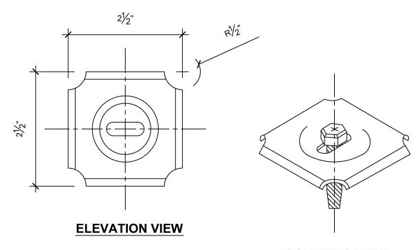
NOTE: MATERIAL IS HOT ROLLED PICKLED AND OILED STEEL (ASTM A569) 1/32" DIA. TYPICAL
